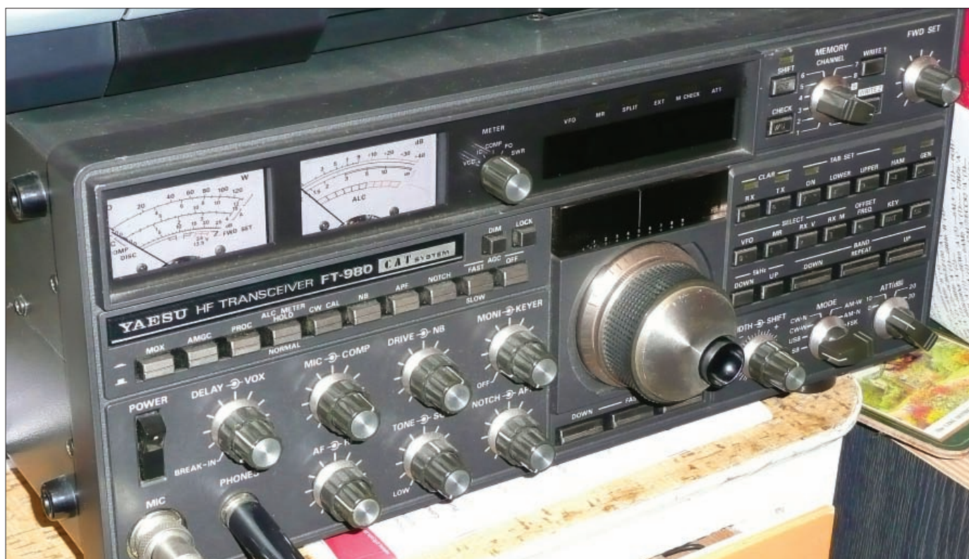
The Yaesu FT-980 rig has very expensive transistors that needed replacing in pairs.
